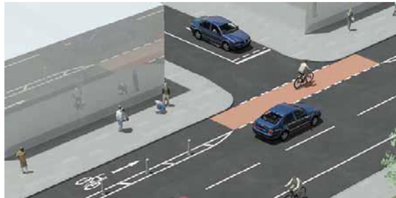
Figure 32: On-Road Cycle Lane Priority Junction Treatment
